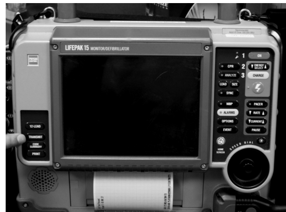
Physio Control Lifepak Model: Manual Defibrillator Operator chooses energy level
